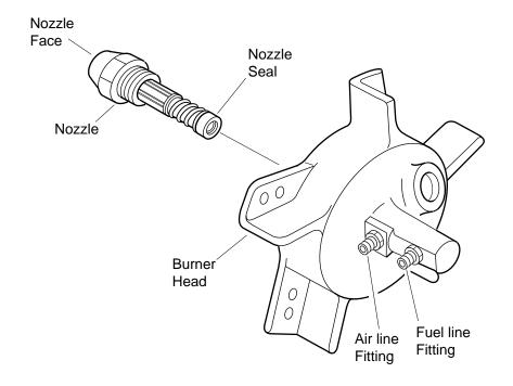
Figure 15 - Removing Nozzle, 100,000 BTU/Hr Model
